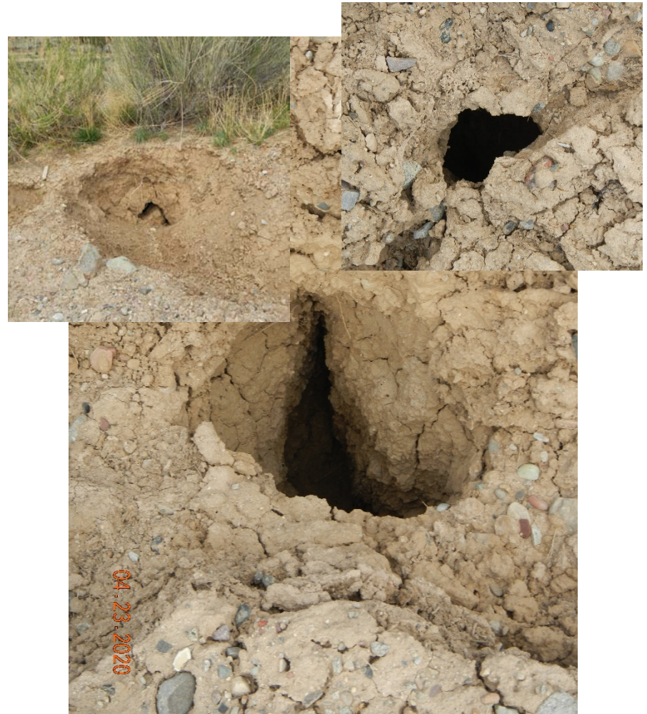
Photo#3: Erosion tunneling.
