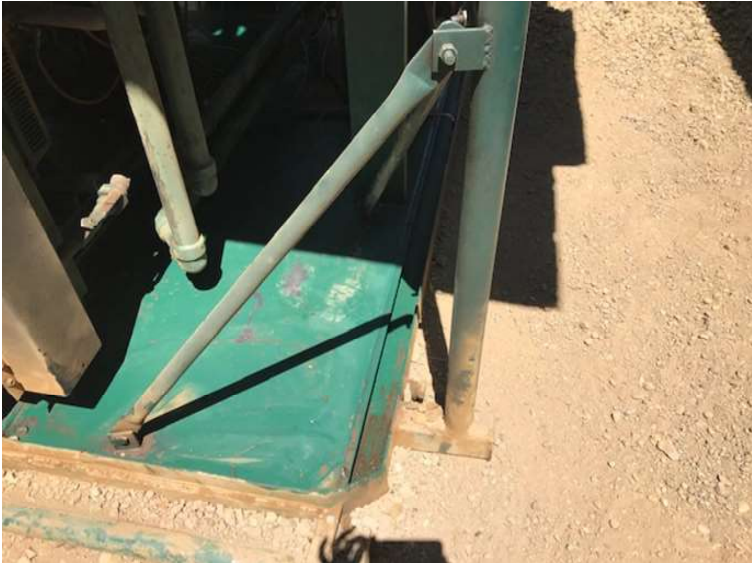
PHOTO 4: THE FLUID ACCUMULATION WAS REMOVED FROM THE LIQUID RING COMPRESSOR SKID AND RESERVOIR. THE IMPACTED SOIL/GRAVEL NEXT TO THE LIQUID RING COMPRESSOR WAS REMOVED FROM THE LOCATION.
