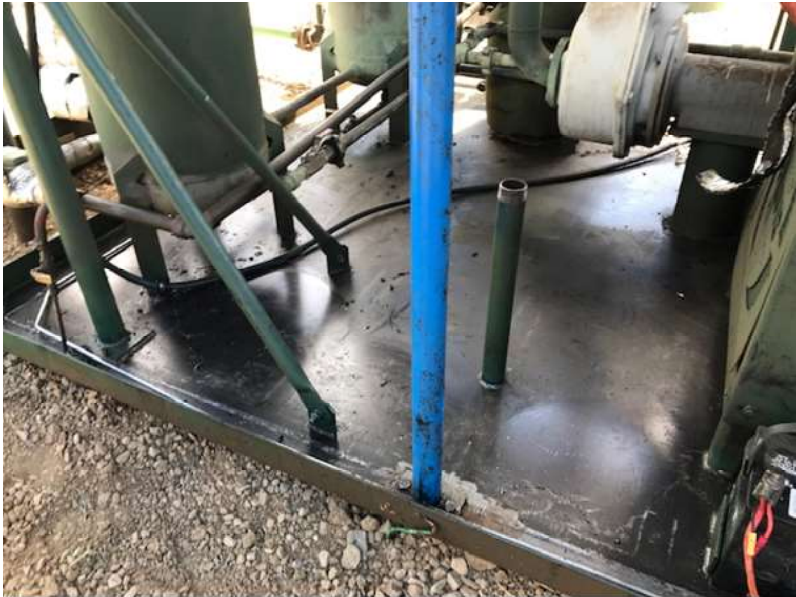
PHOTO 3: THE FLUID ACCUMULATION WAS REMOVED FROM THE LIQUID RING COMPRESSOR CONTAINMENT SKID. THE IMPACTED SOIL/GRAVEL NEXT TO THE LIQUID RING COMPRESSOR WAS REMOVED FROM THE LOCATION. CONTAINMENT WAS CLEANED UP.
