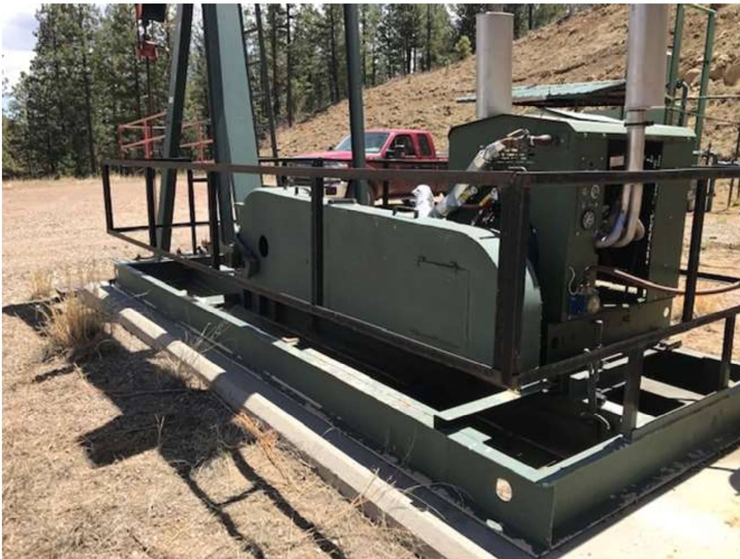
PHOTO 3: THE BELT GUARD HAD BEEN REMOVED FROM THE PUMPING UNIT FOR MAINTENANCE TO THE CLUCH. THE BELT GUARD WAS PLACED BACK ON THE UNIT.
