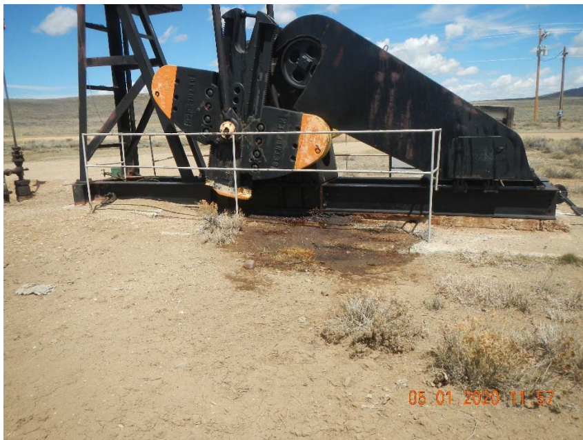
Photo 3. Stained soil at pump jack motor.
