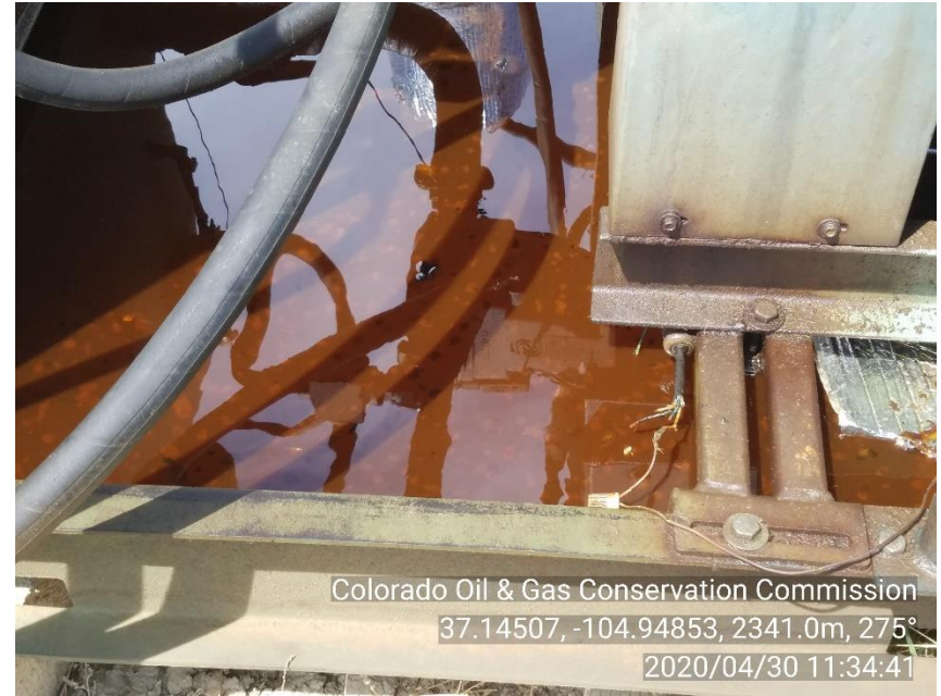
PHOTO 4: STANDING OIL IN PRIME MOVER ENGINE SKID. APPEARS THAT ENGINE OIL IS BEING DRAINED INTO SKID. Comply with general provisions of the oil and gas act for wildlife protection. ENGINE SKID IS FULL OF FLUID AND ABOUT TO RUN OVER 24 OURS TO CORRECT CA DATE 5-1-20.
