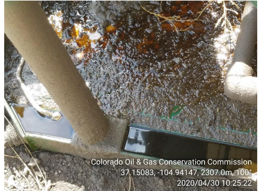
PHOTO 4: STANDING OIL IN COMPRESSOR SKID. Comply with general provisions of the oil and gas act for wildlife protection. CA DATE 5-7-20.
