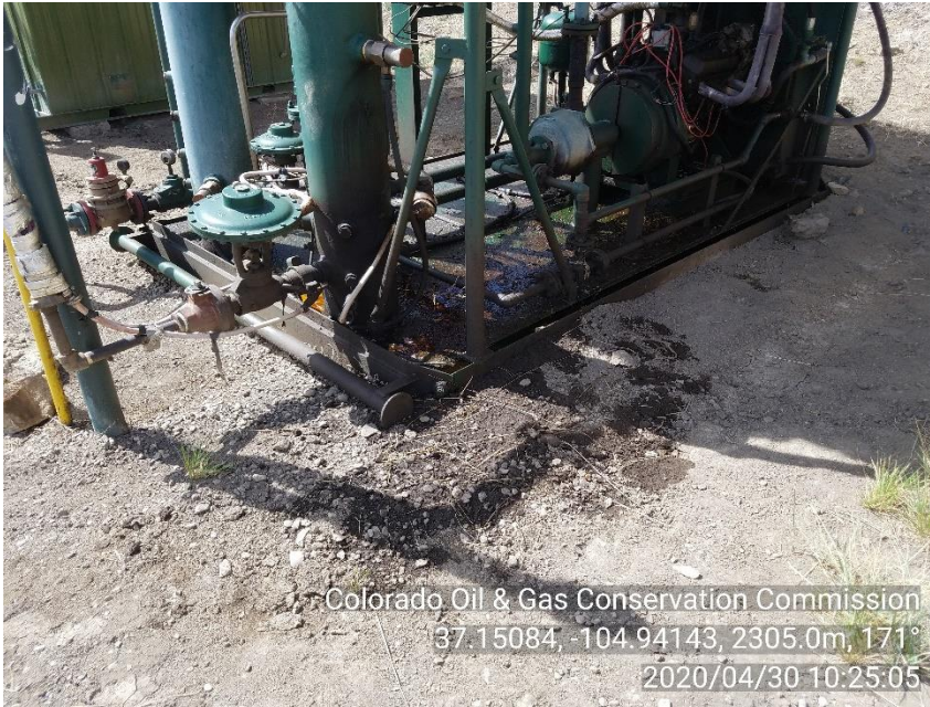
PHOTO 3: Stained soil around HYD skid. Non E&P Waste not properly stored, handled, transported, treated, or disposed per Rule 907A CA DATE 5-7-20. THIS IS SECOND NOTICE FOR THIS CORRECTIVE ACTION.
