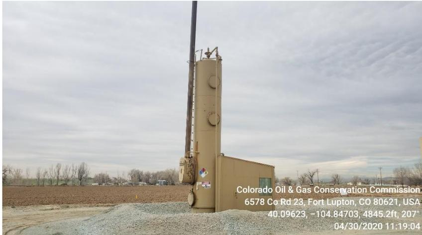
**Photo 7 Vertical Heated separator**
