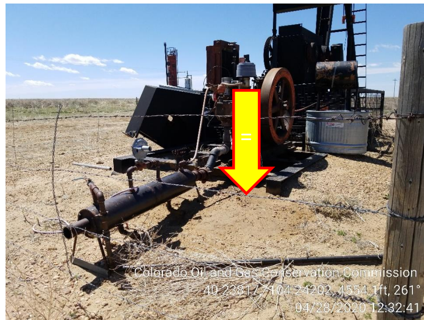
Photo 6 – Stained Soil at Gas Engine
