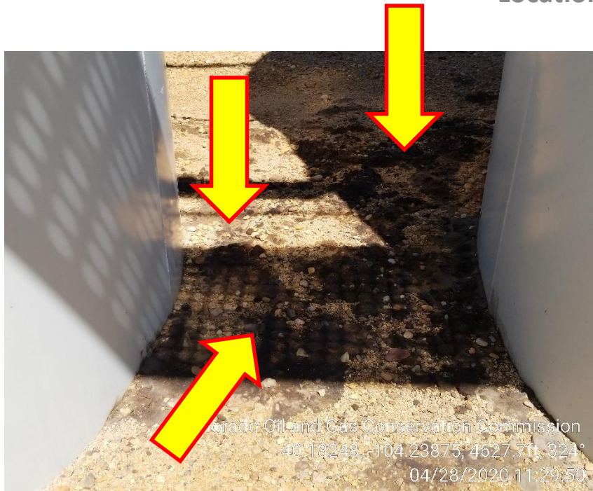
Photo 5 – Stained Soil in between tanks
