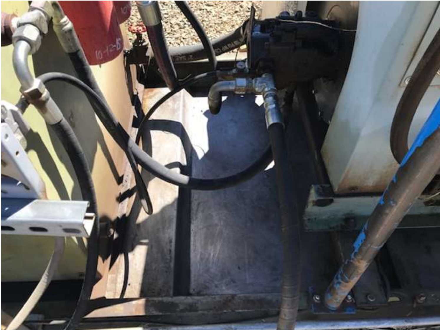
PHOTO 2: THE FLUID ACCUMULATION IN THE CONTAINMENT BELOW THE ENGINE WAS REMOVED AND THE SKID WAS CLEANED UP.
