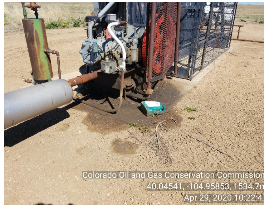
Photo 2 Stained soil around PU motor and Mechanical issue
