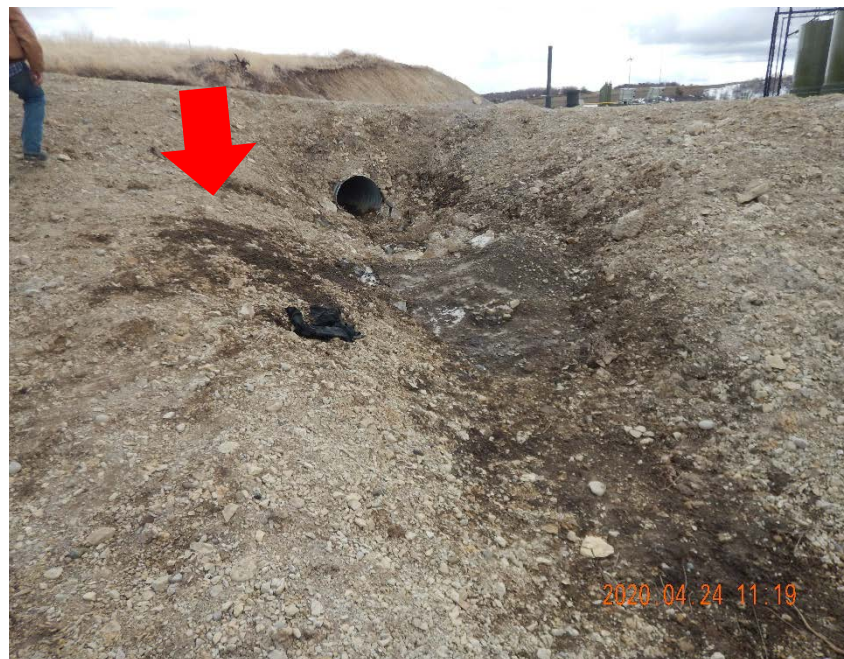
Photo #11 – Trash and stained soil located beneath culvert at north end of pad. Hydrocarbon odors were observed in the dark soil at this location (red arrow). Operator was notified of this issue via phone on 4/24/2020.
