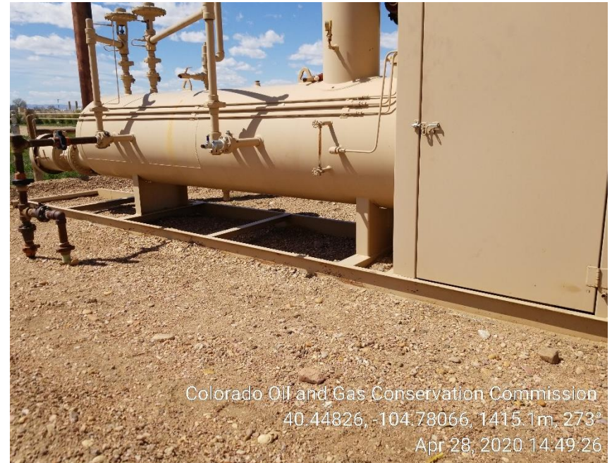
Photo 6: Separator not anchored
