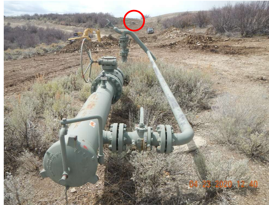
View of the pig chute and valve can (red circle) where the 4-inch pipeline was installed
