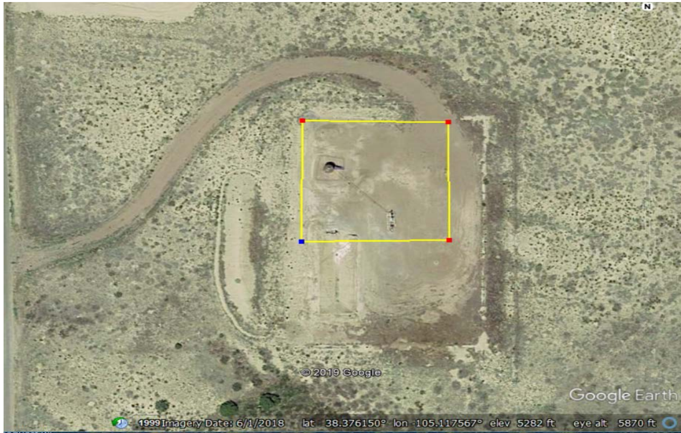
Photo 7. Aerial image shows the location and the outline shows approximately the size of the location it should be reduced to. Unused areas of the location must be reclaimed.
