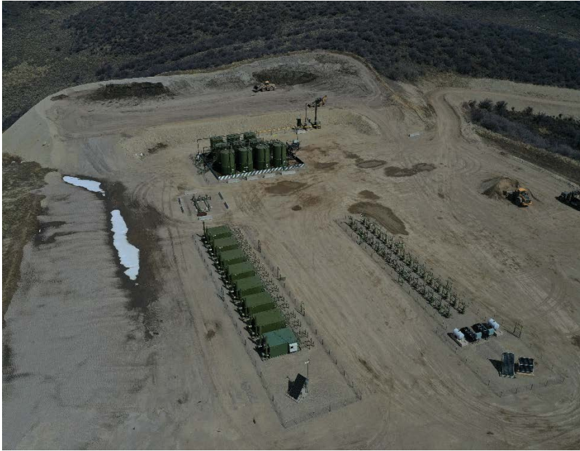
Photo #1 – Overview of pad from southwest. Note treated drill cuttings have been applied on west and north sides of pad. Localized accumulations of oil-stained soil observed along west side of pad
