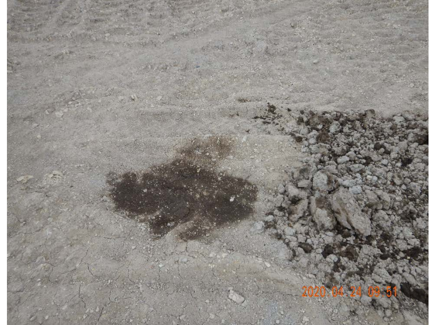
Photo #12 - Localized accumulation of oil-stained soil on west side of pad. (5)
