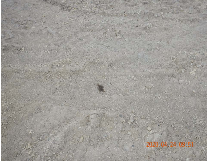
Photo #13 - Localized accumulation of oil-stained soil on west side of pad. (6)
