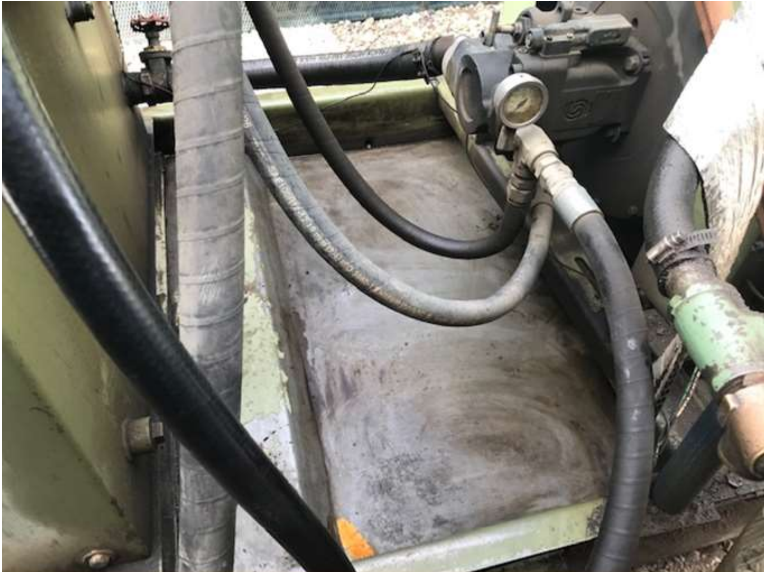
PHOTO 4: THE FLUID ACCUMULATION IN THE PC ENGINE SKID FOR GE 28-07 WAS REMOVED AND THE SKID WAS CLEANED UP.
