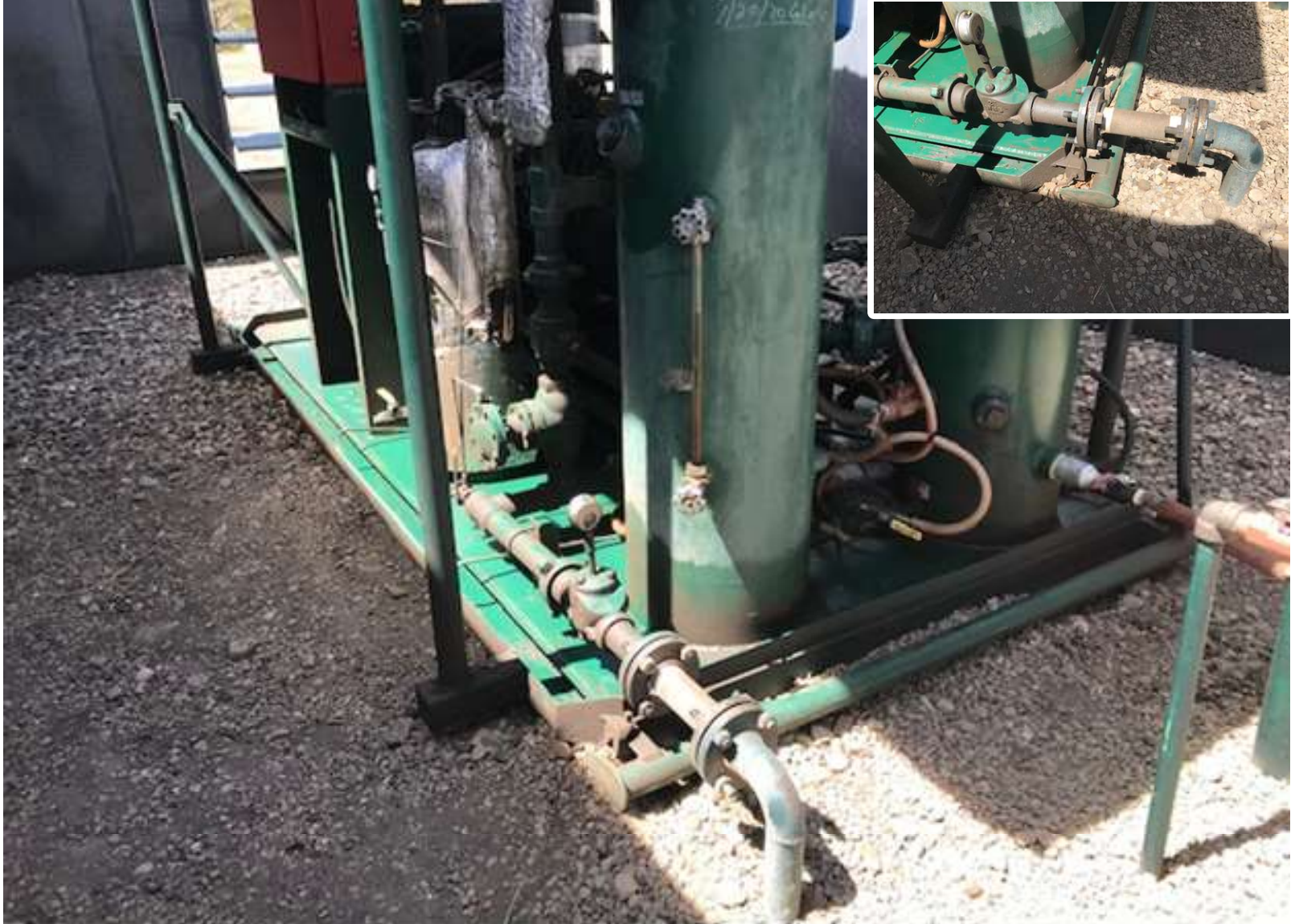
PHOTO 3: THE IMPACTED SOIL/GRAVEL SURROUNDING THE GE 28-07 LIQUID RING COMPRESSOR WAS REMOVED FROM THE LOCATION. THE SKID AND RESERVOIR WAS CLEANED UP
