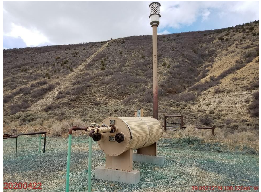
Photo 20: Photo taken from the northwest end of the Location, facing west. Photo shows unused/abandoned equipment (heater treater) on Location. All unused/abandoned equipment requires removal in accordance with Rule 603.f
