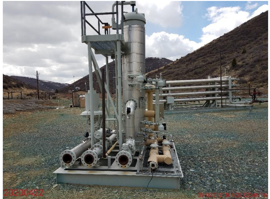
Photo 60: Photo taken from the southeast end of the Location, facing south. Photo show an unused Coalescing Filter stored on the Location. Filter missing blind flange ends; flanges are required to be placed on filter immediately.
