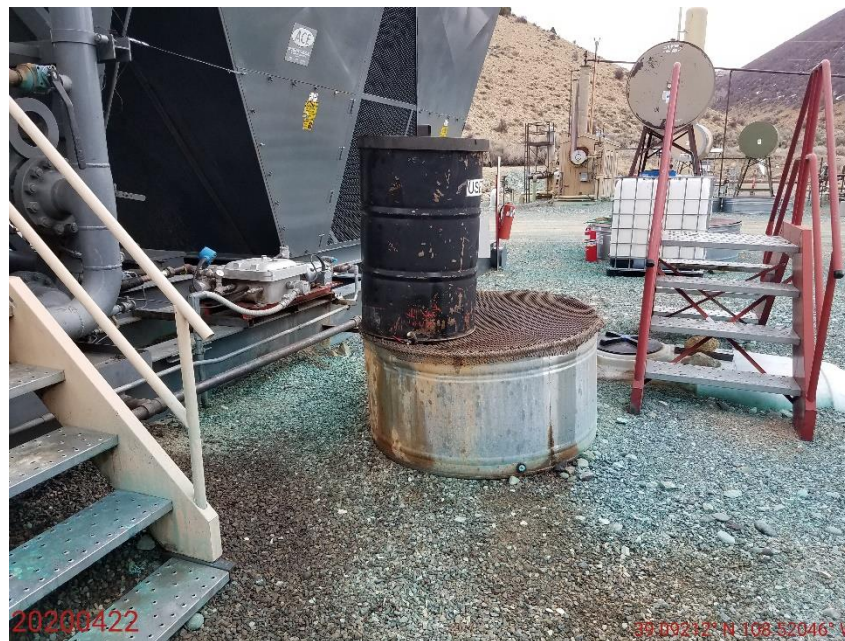
Photo 44: Photo taken from the compressor on the west end of the Location. Photo shows barrel of oil placed upon secondary containment. Photo also shows stained soils on Location.
