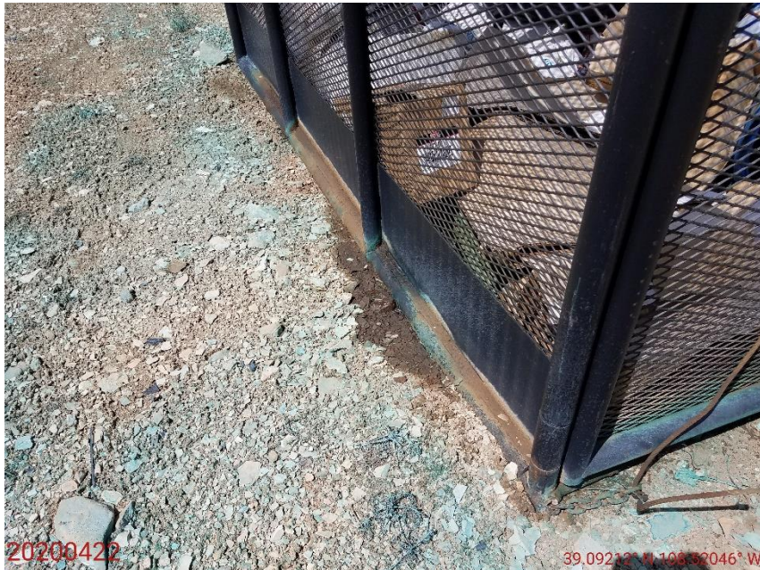
Photo 77: Photo taken from the trash container. Photo shows stained soils; oily chemicals appear to be discharging from the trash container.
