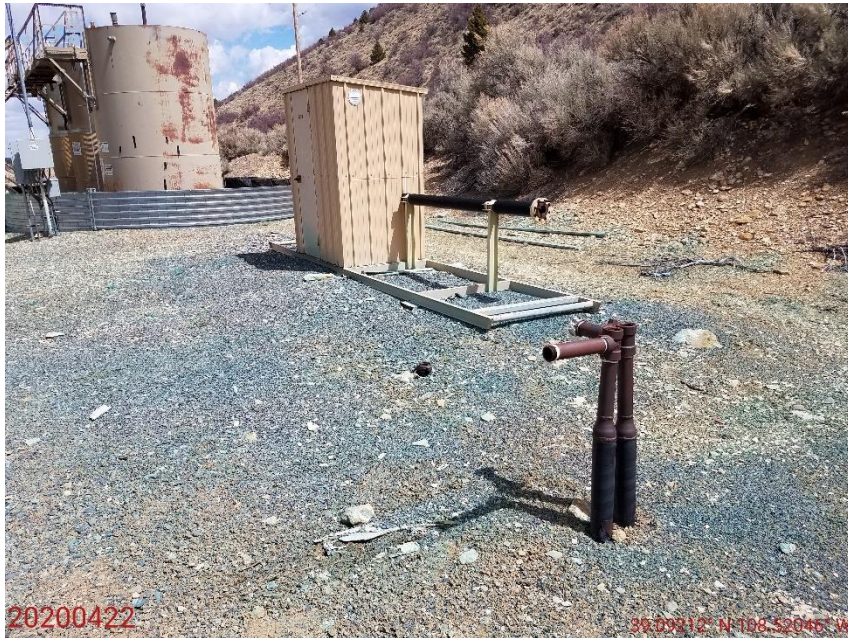
Photo 71: Photo taken from the east end of the Location, facing northeast. Photo shows unused/abandoned equipment (meter shed, risers) on Location, with stones placed upon the open pipe; this is improper capping procedure. All unused/abandoned equipment requires removal in accordance with Rule 603.f.
