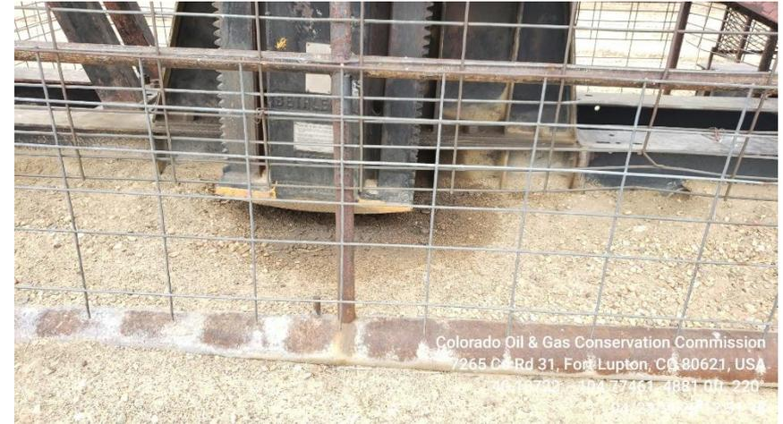
**Photo 3 Stained soil under pump jack counter weights**
