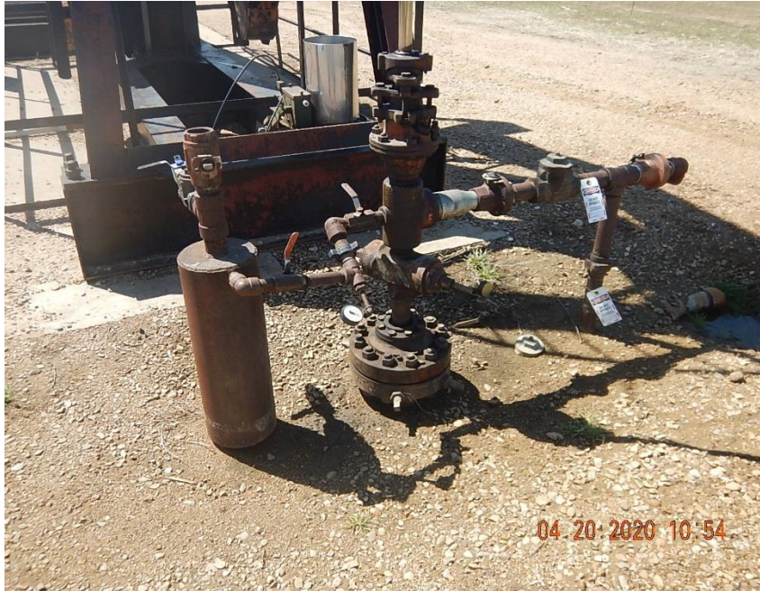
View of Nessu #1 wellhead (API 123-07762); OOSLAT (flowline shut in/ tagged out)
