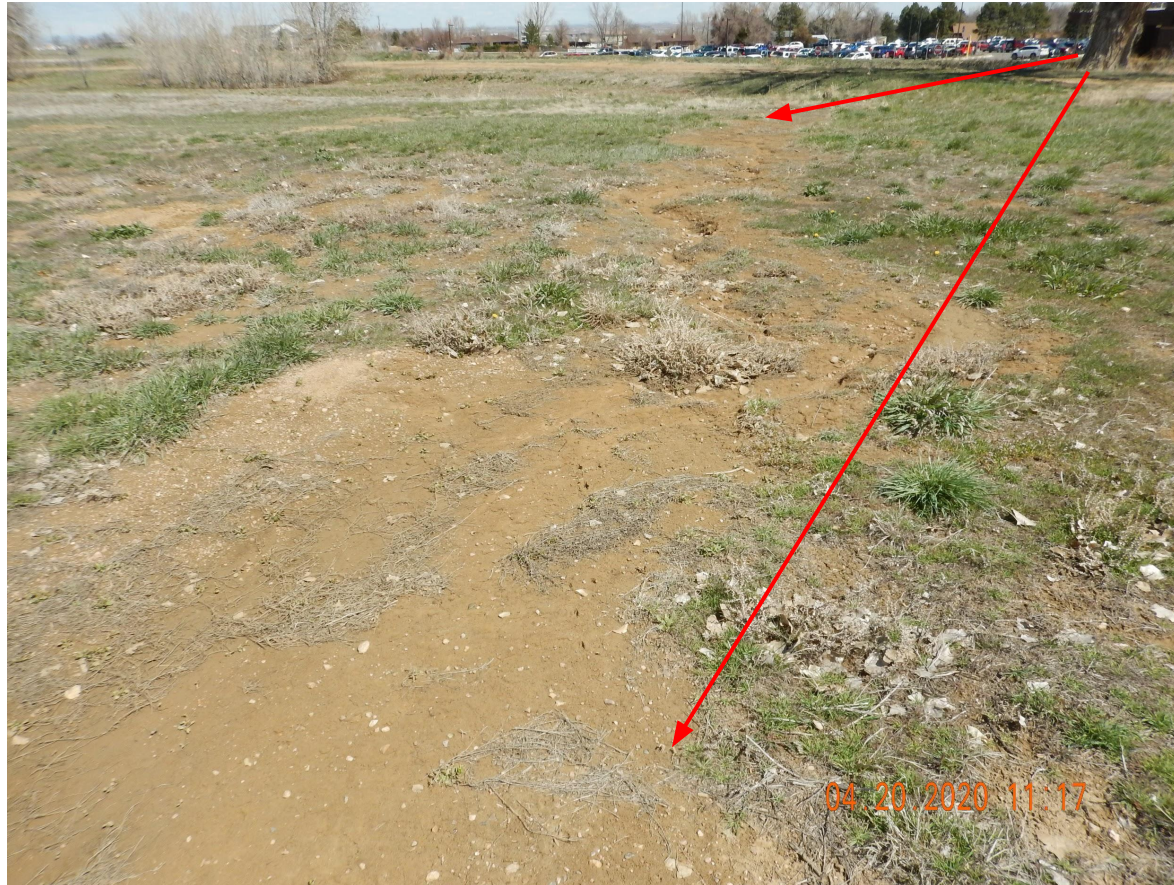
Photo 2. Photo taken from the northern location, facing North. Photo illustrates erosion and sediment discharge off location.
