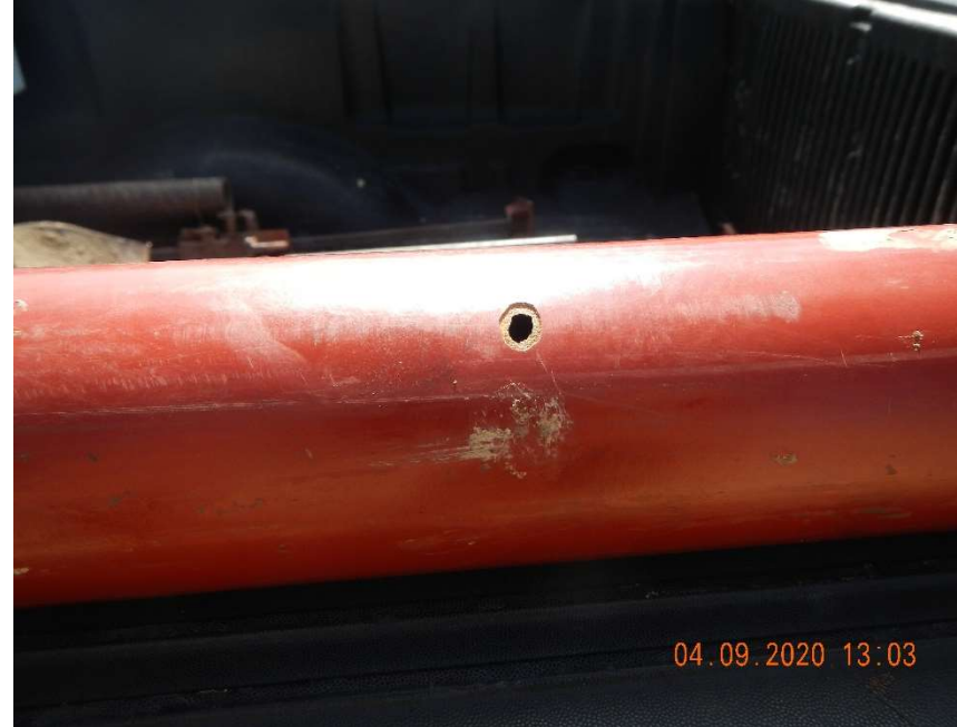
Cut out section of the flowline that failed the pressure test.
