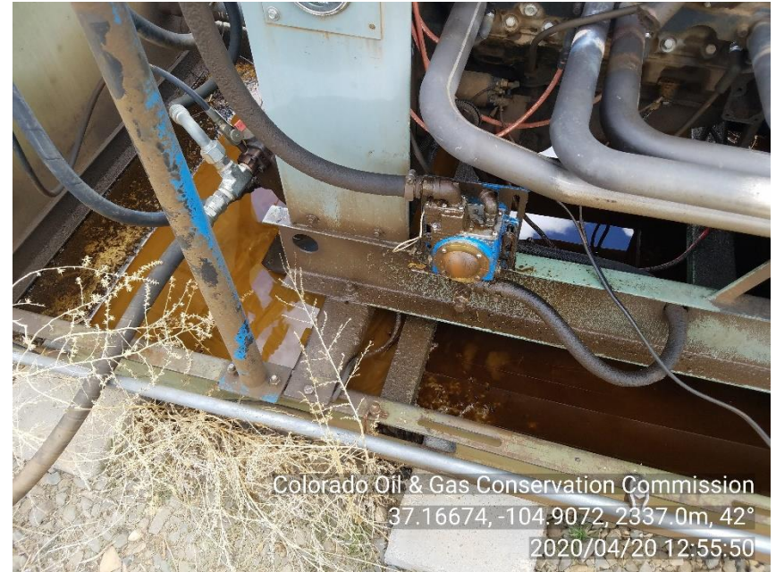
PHOTO 4: THERE IS STANDING OIL IN ENGINE SKID. Comply with general provisions of the oil and gas act for wildlife protection. CA DATE 5-20-20
