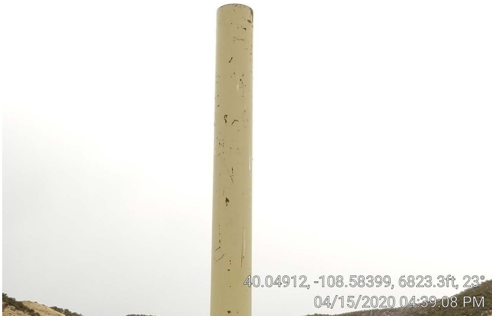
Photo 8. Tank stack without bird protection.
