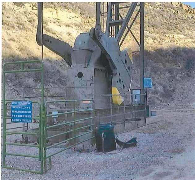
MG # 18 Well location with tubing removed
