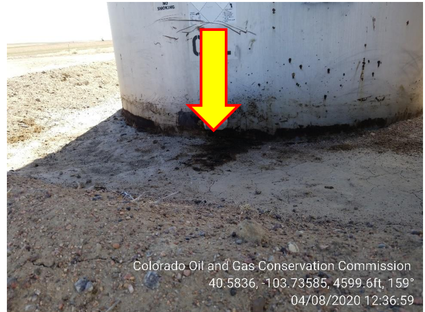
Photo 6 – Stained Soil at NE Loadline
