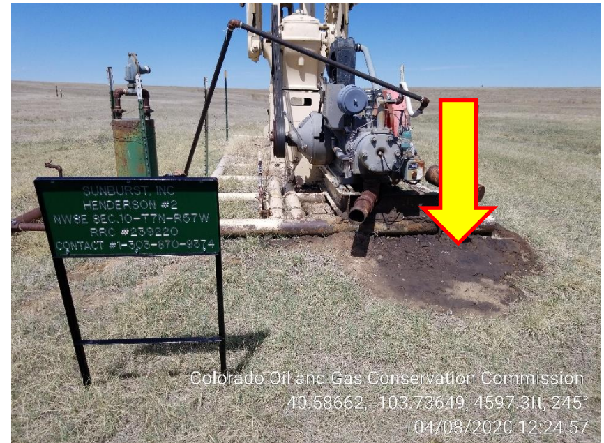
Photo 2 – Stained Soil at Gas Engine
