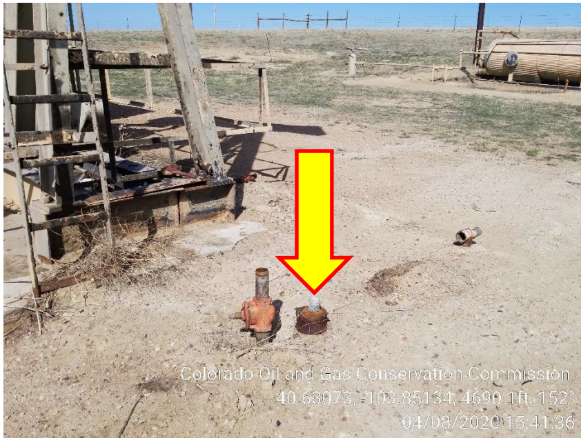
Photo 3 – Well has been Plugged and Abandoned. Open Well Bore has been covered at Surface
