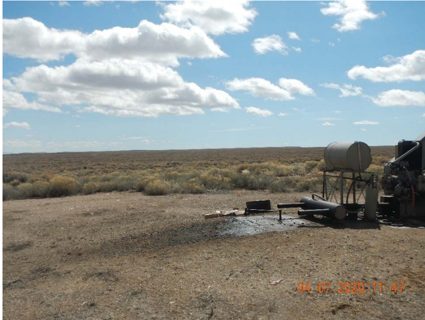
Photo 2. Stained soil at pump jack.
