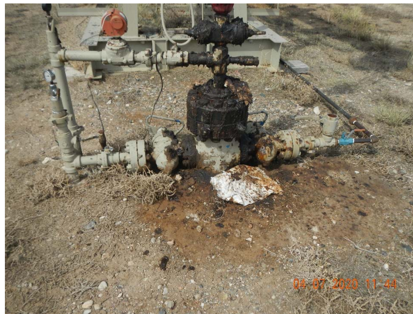
Photo 3. Stained soil at wellhead.
