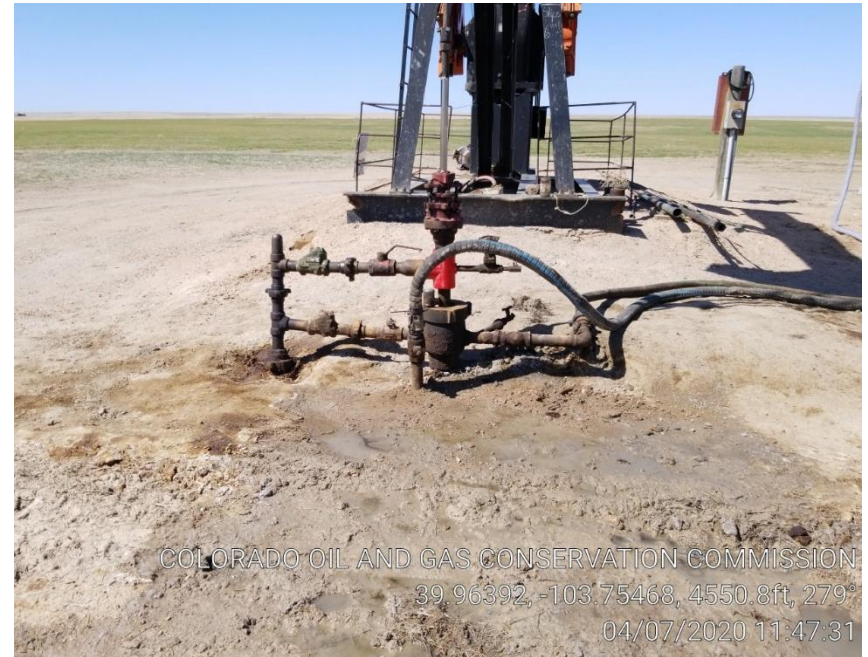
Pic 4 leaking wellhead
