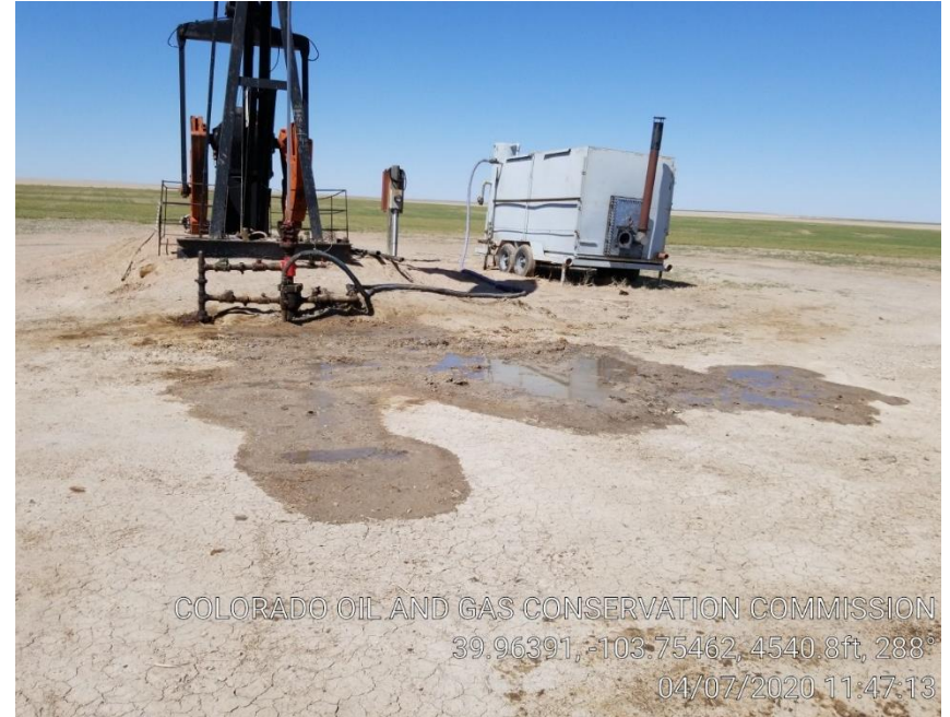
Pic 2 leaking wellhead
