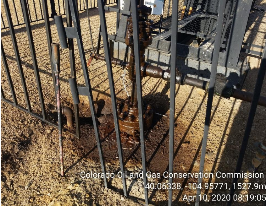
Photo 3 Mechanical issue and stained soil around well head
