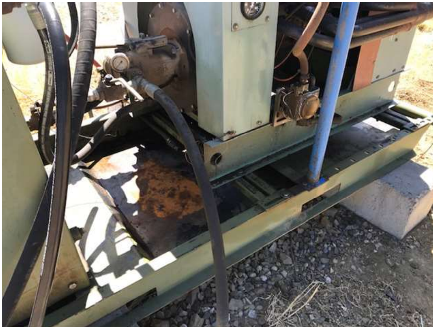
PHOTO 7: THE FLUID ACCUMULATION WAS REMOVED FROM THE PC ENGINE SKID.
