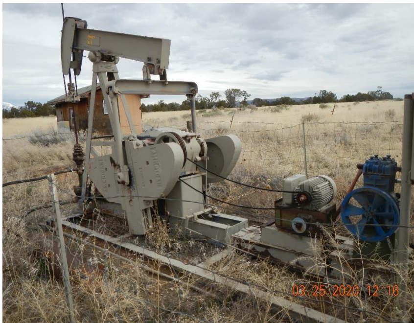
Hall #1 pump jack and electric prime mover.
