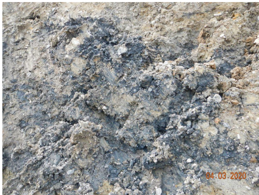
Photo#11: Close up of stained soil on pit wall.
