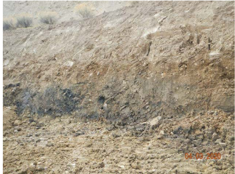
Photo#9: West Pit wall, accumulation of stained soil.
