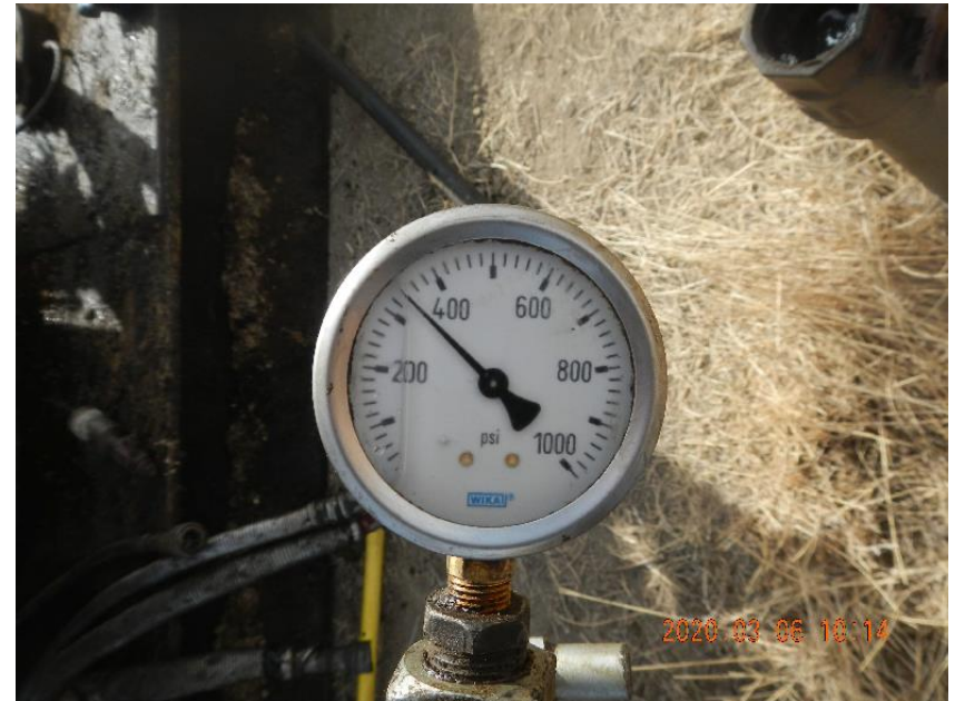
Photo 2: Passed pressure test reading.
