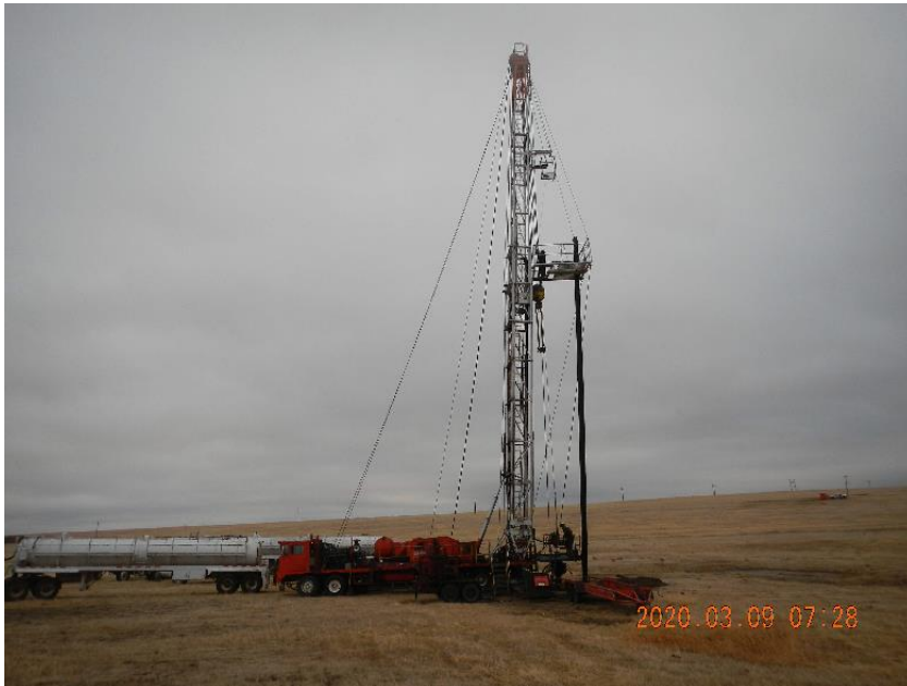
Photo 3: Tubing tripped out of well and standing in the derrick.
