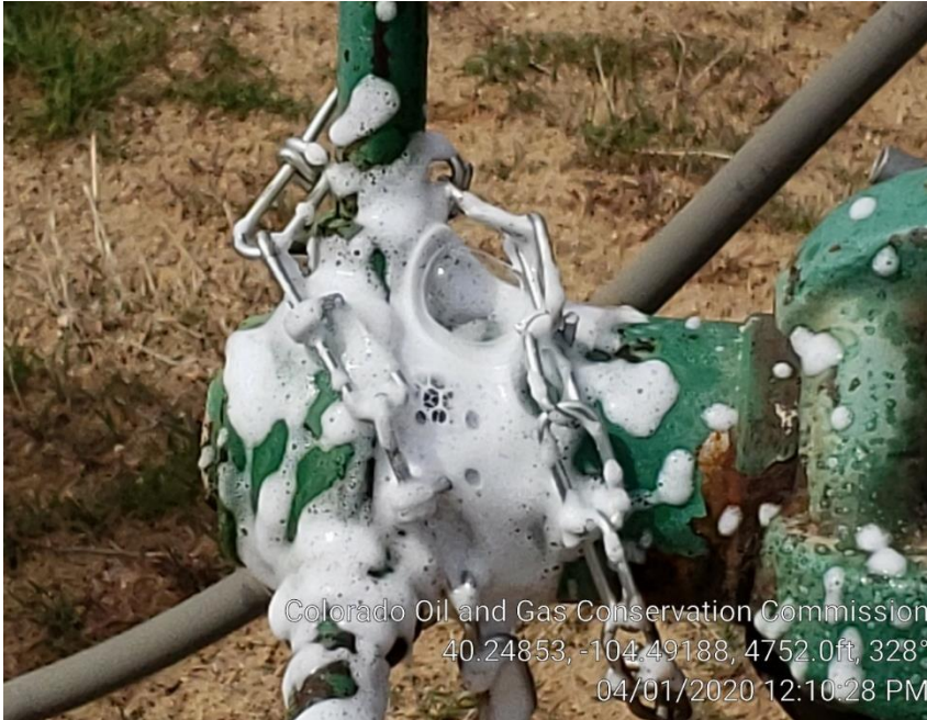
Photo #3 Leaking gas
