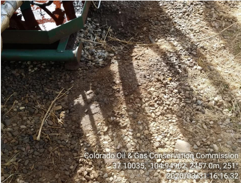
PHOTO 3: AREA OF IMPACTED SOIL APPEARS TO BE FROM DRAINING COMPRESSOR SKID ON THE GROUND. Conduct maintenance on equipment, cleanup stained material and review self inspection processes. CA DATE 4-30-20.
