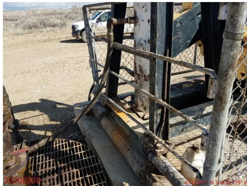
Photo 4: Photo taken from the wellhead. Inspection #696201101 documented venting from an open valve on equipment attached to the bradenhead. Valve appears to have been closed and well is no longer venting.
