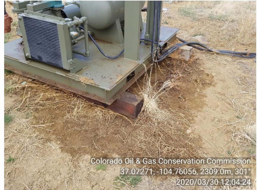
PHOTO 6: IMPACTED SOIL AROUND COMPRESSOR APPEARS TO BE HYDRALIC OIL FROM COMPRESSOR. Conduct maintenance on equipment, cleanup stained material and review self inspection processes. CA DATE 4-30-20
