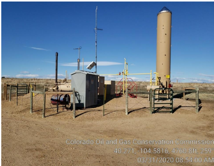
Photo #2 Separator, ECD & Meter Run
