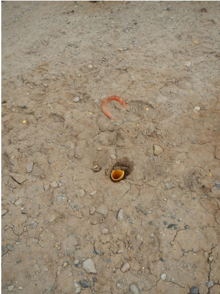
Photo#4: Unmarked, damaged Anchor.
