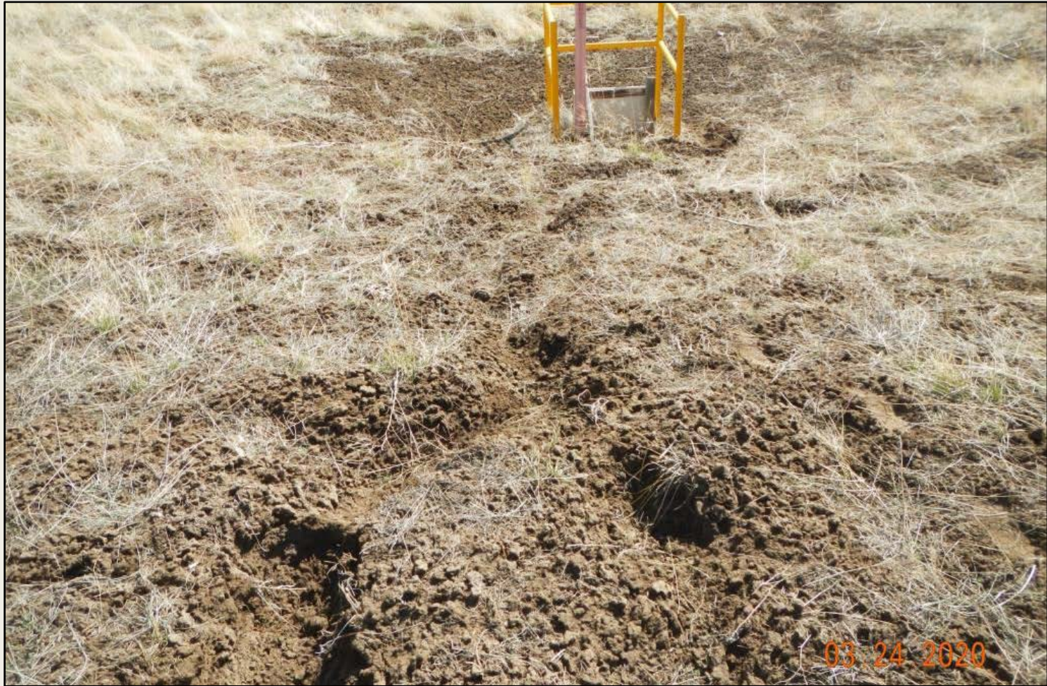
Photo 3. View of erosional channel channeling approximately 1 foot wide and 10 inches deep, within the southwestern project area.
