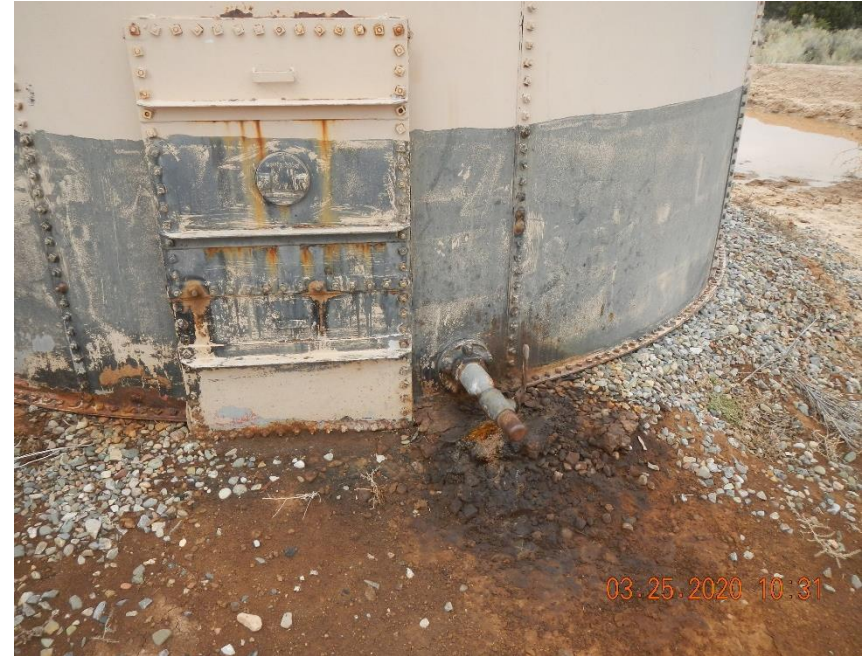
Oil stained soil beneath load out valve.
