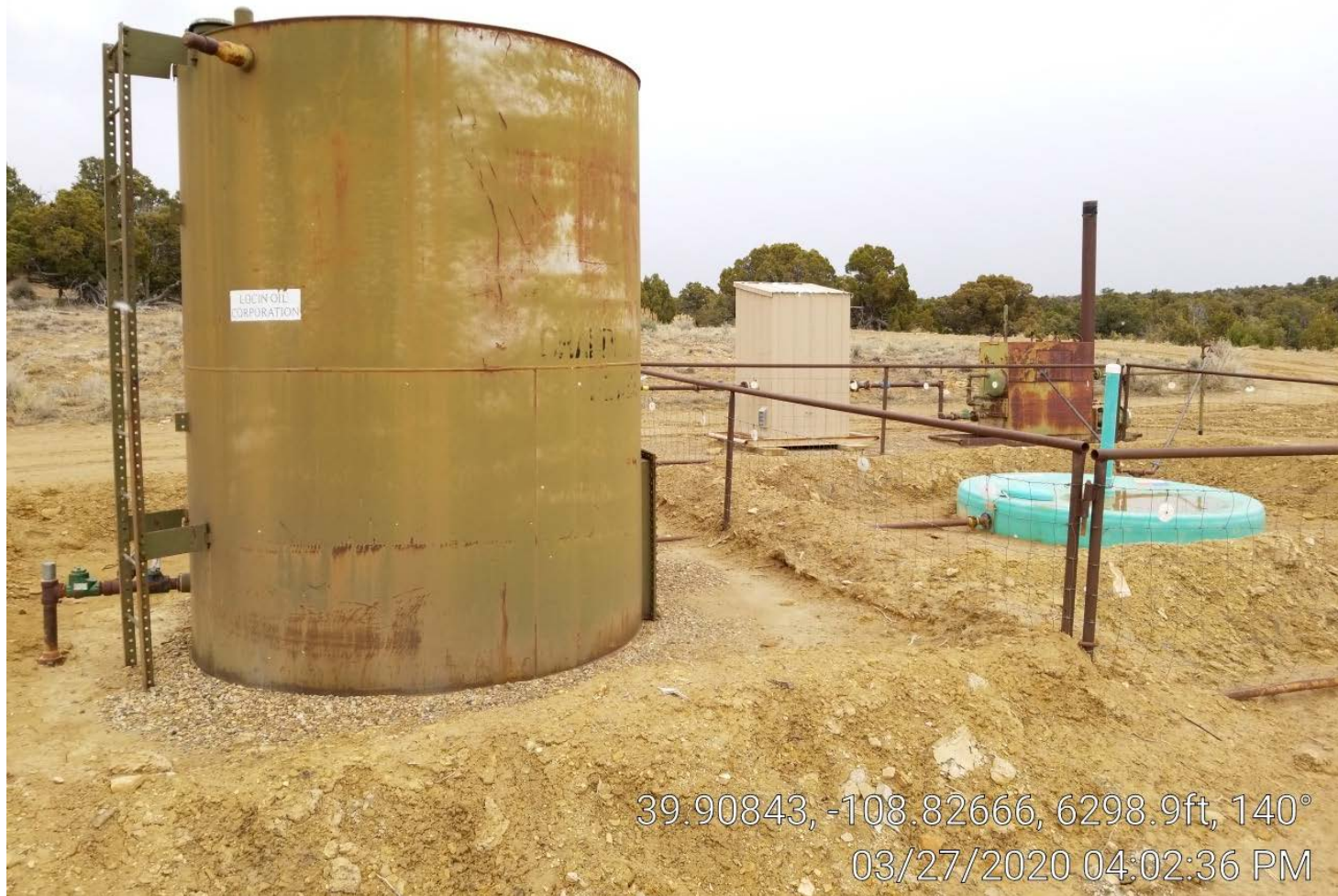
Photo 3. Tanks, meter building, and separator.
