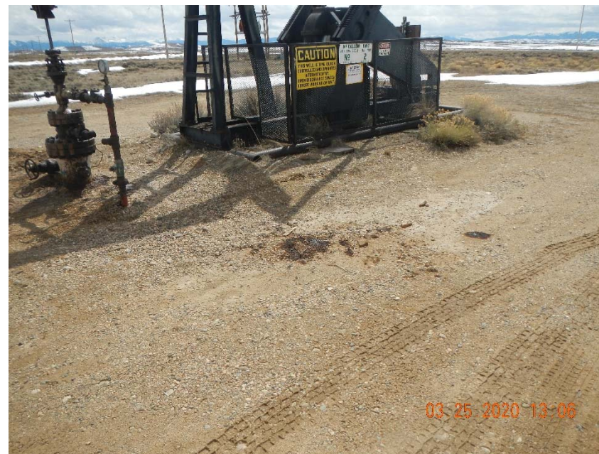
Photo 2. Stained soil at wellhead.
