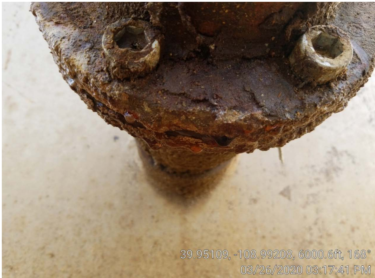
Photo 6. Leaking tank flange.
