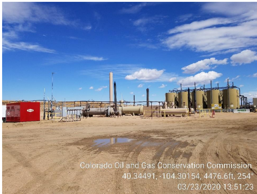
Photo 3 – Tank Battery
