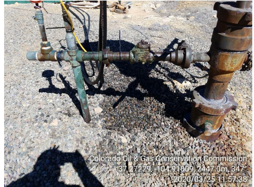
PHOTO 4: AREA OF IMPACTED SOIL NEAR WELLHEAD APPEARS TO BE COMING FROM HYDRAULIC HOSE. Non E&P Waste not properly stored, handled, transported, treated, or disposed per Rule 907A. CA DATE REMAINS THE SAME DATE ON THE ORIGINAL INSPECTION DOC#695102044.
